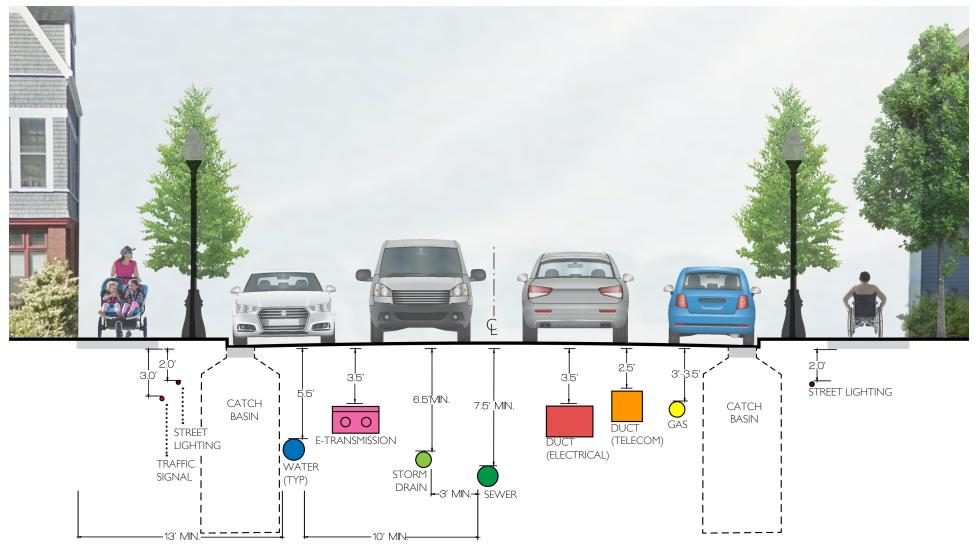
NOTE: ALL DIMENSIONS TO BE IMPLEMENTED UNLESS OTHERWISE APPROVED BY PWD. UTILITIES MAY NEED TO OFFSET AROUND MANHOLES & CATCH BASINS. IF NEEDED, E- TRANSMISSION CAN GO UNDERNEATH ELECTRICAL DUCT.
