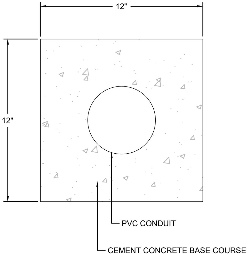
NOTE: PVC CONDUIT SHALL BE ENCASED IN 12 INCHES OF CEMENT CONCRETE BASE COURSE. SAND WILL NOT BE REQUIRED AT THESE LOCATIONS. CONCRETE WILL BE PAID FOR UNDER ITEM 431.1, HIGH EARLY STRENGTH CEMENT CONCRETE BASE COURSE.
