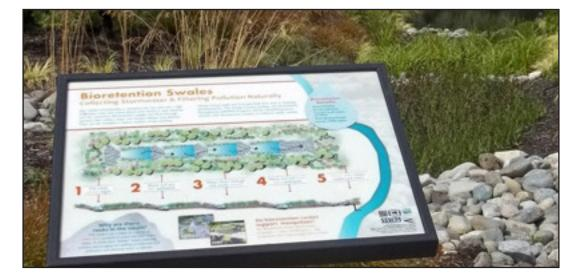
Cleverly disguised as beautiful park feature, this bio-retention pond will serve both form and function as a low-impact stormwater device. Pathways around the pond will include interpretive infrastructure displays to point out how the North Dorchester CSO Tunnel and Columbia Road Headworks Facility (nearby MWRA Facilities) keep Carson Beach clean and protect public health in the community.
