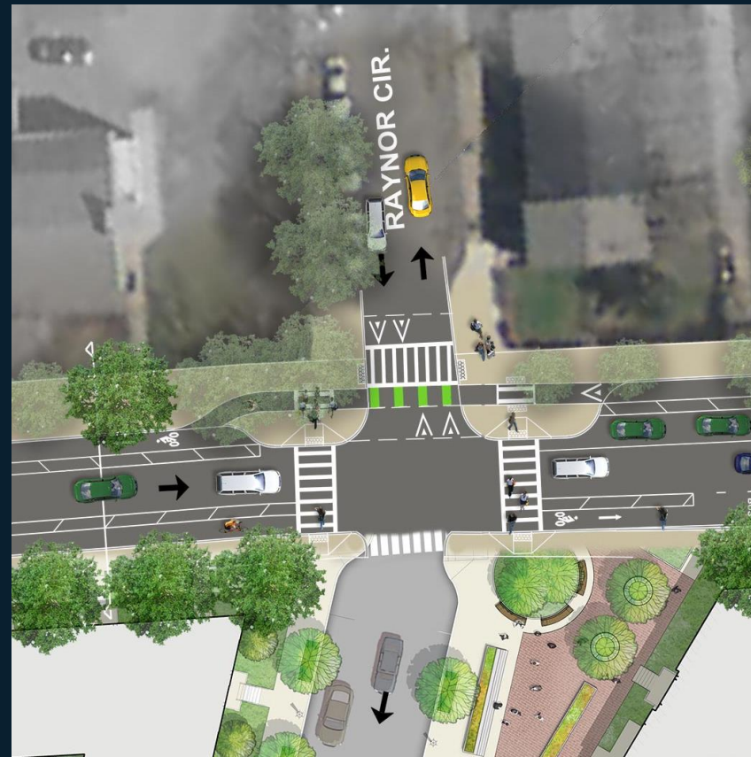
Curb Extensions Raised Crosswalk Narrowed Travel Lanes
