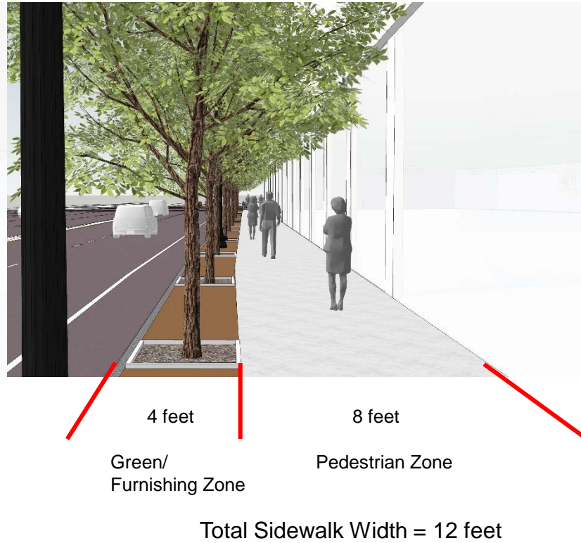
Recommended width, typical sidewalk
