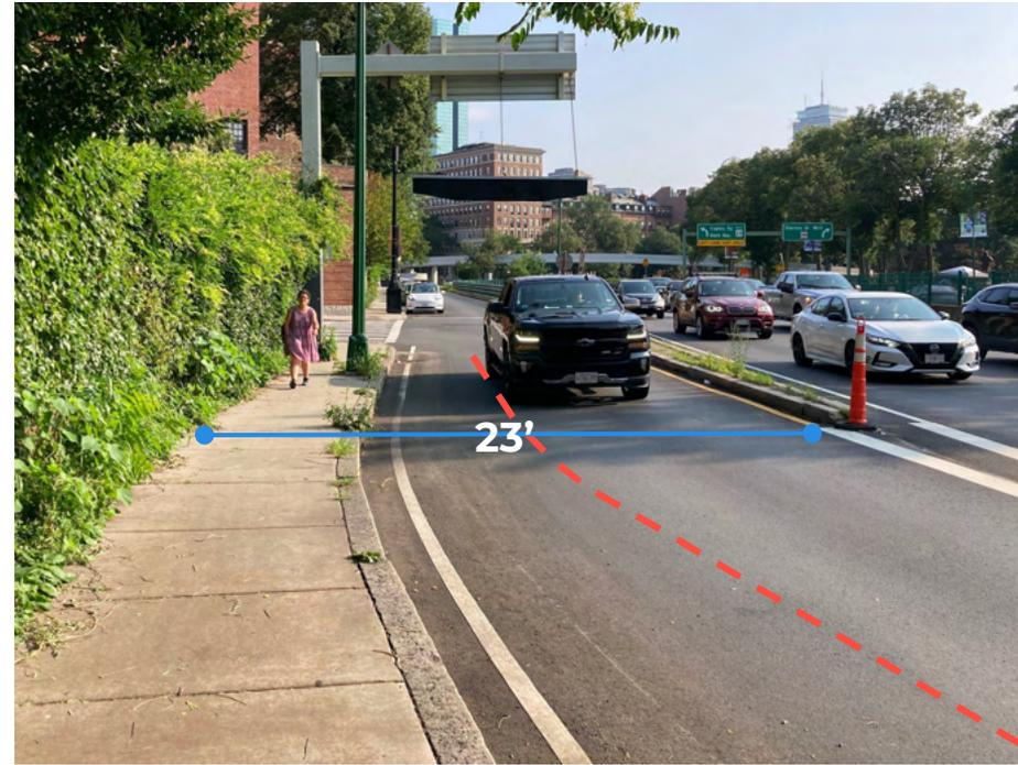
Above: a red dashed line shows where the approximate edge of a 10 foot wide path would be. A blue solid line shows the narrowest constrained dimension in the Storrow onramp area.
