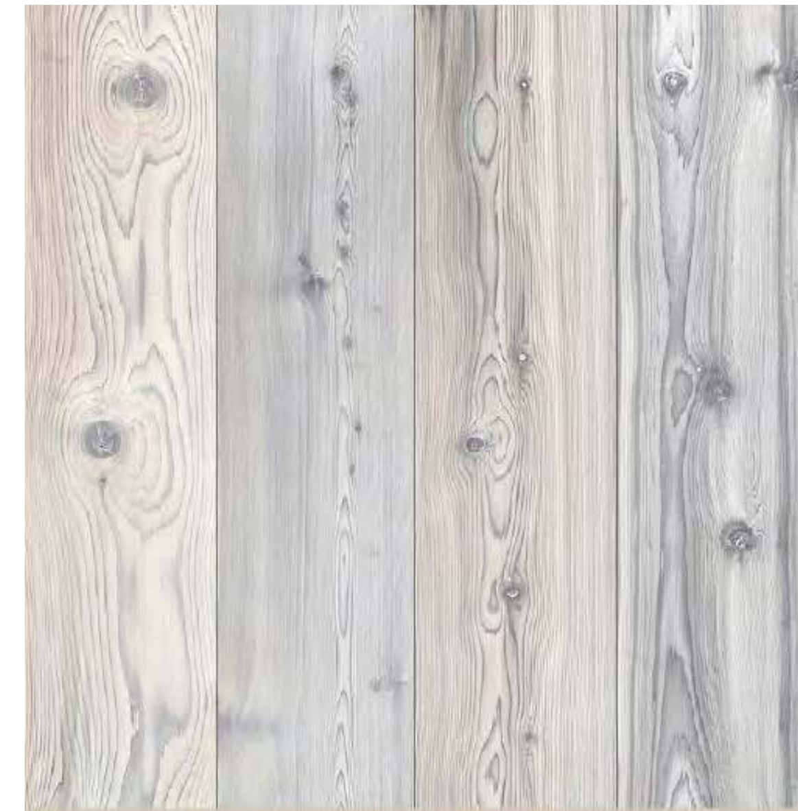
05 ROOF TOP - INSPIRED MATERIAL FOR WALL WEATHERED ALASKAN YELLOW CEDAR / 5"W NOT TO SCALE
