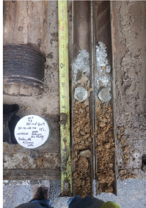
Photo 3: View of sample S-6 from 12 to 14 feet bgs at boring location NB-2.
