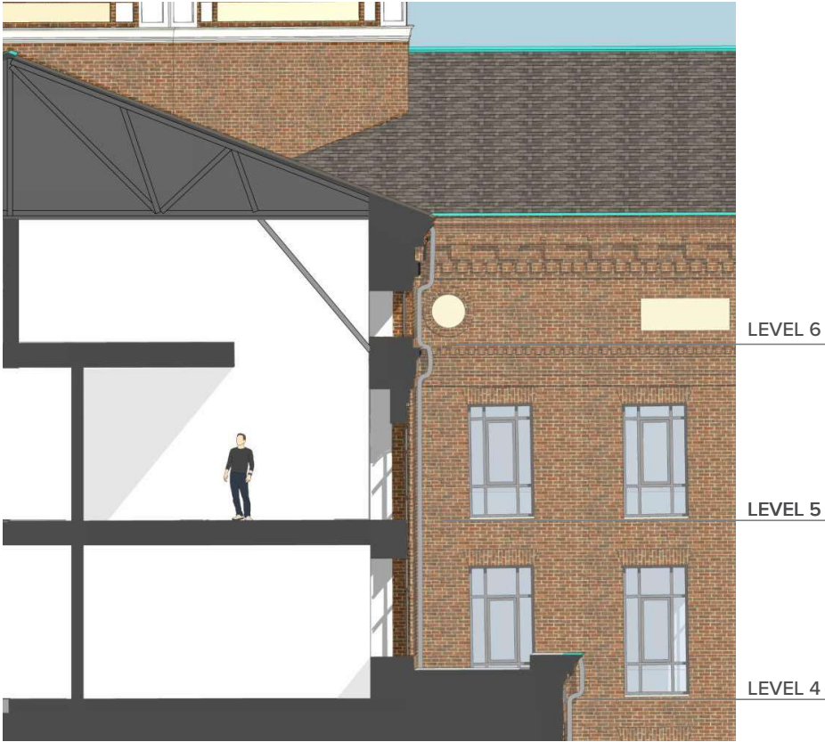
CLERESTORY WINDOW IN LEVEL 5 LOFT UNITS
