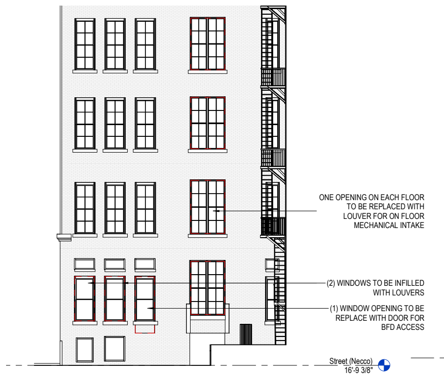
EXISTING ELEVATION - SOUTH DOCK
