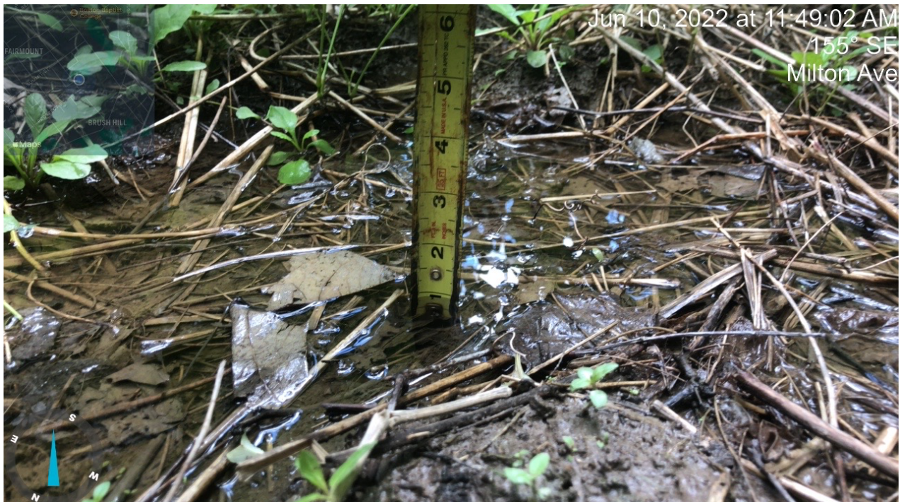
Photo 2: The depth of standing water within the A-series IVW averaged 1 inch during observations made on June 10, 2022.
