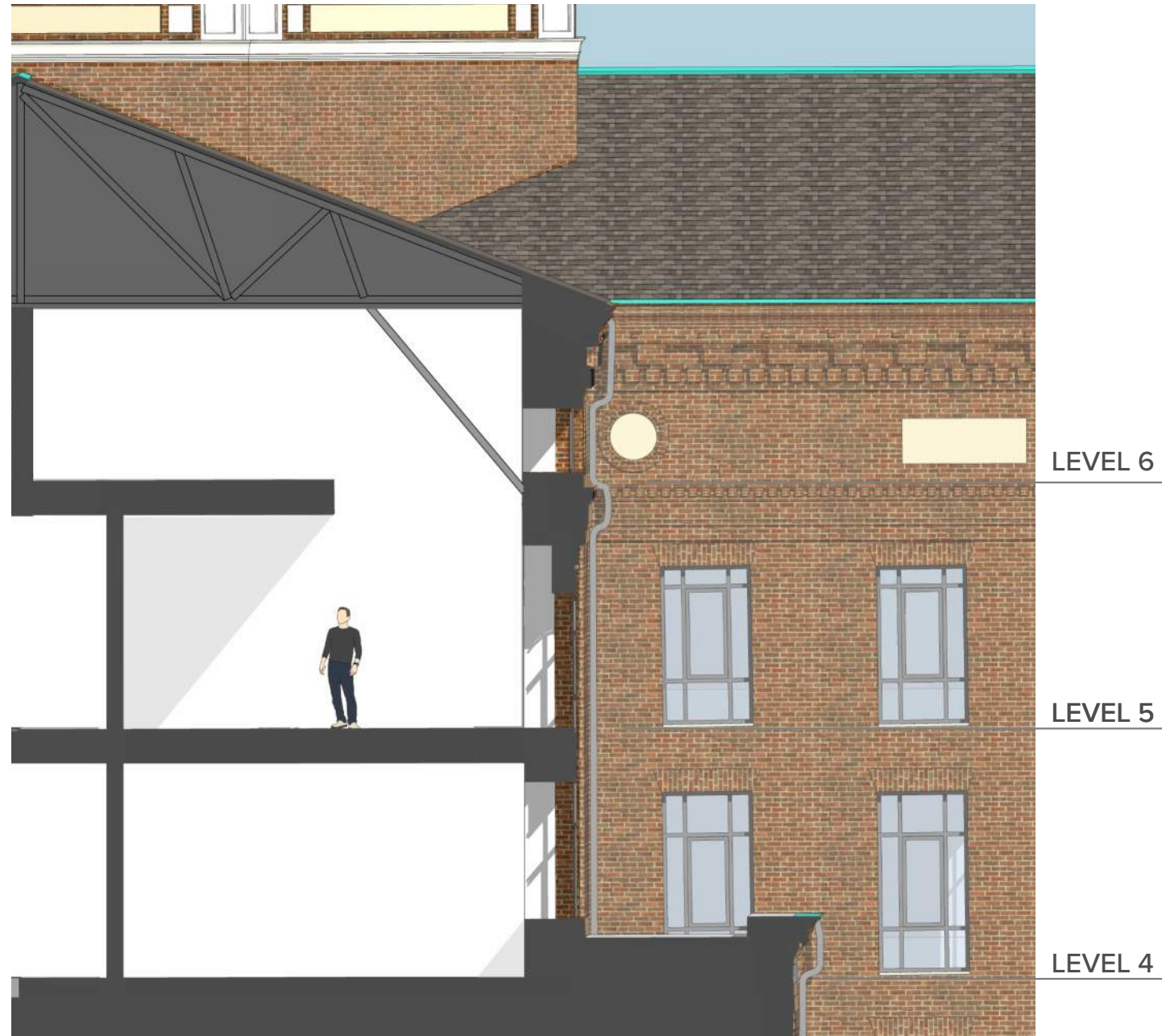
CLERESTORY WINDOW IN LEVEL 5 LOFT UNITS
