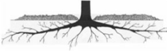
Example of how mulch should be installed. 2-4 inches thick and not against the trunk.
