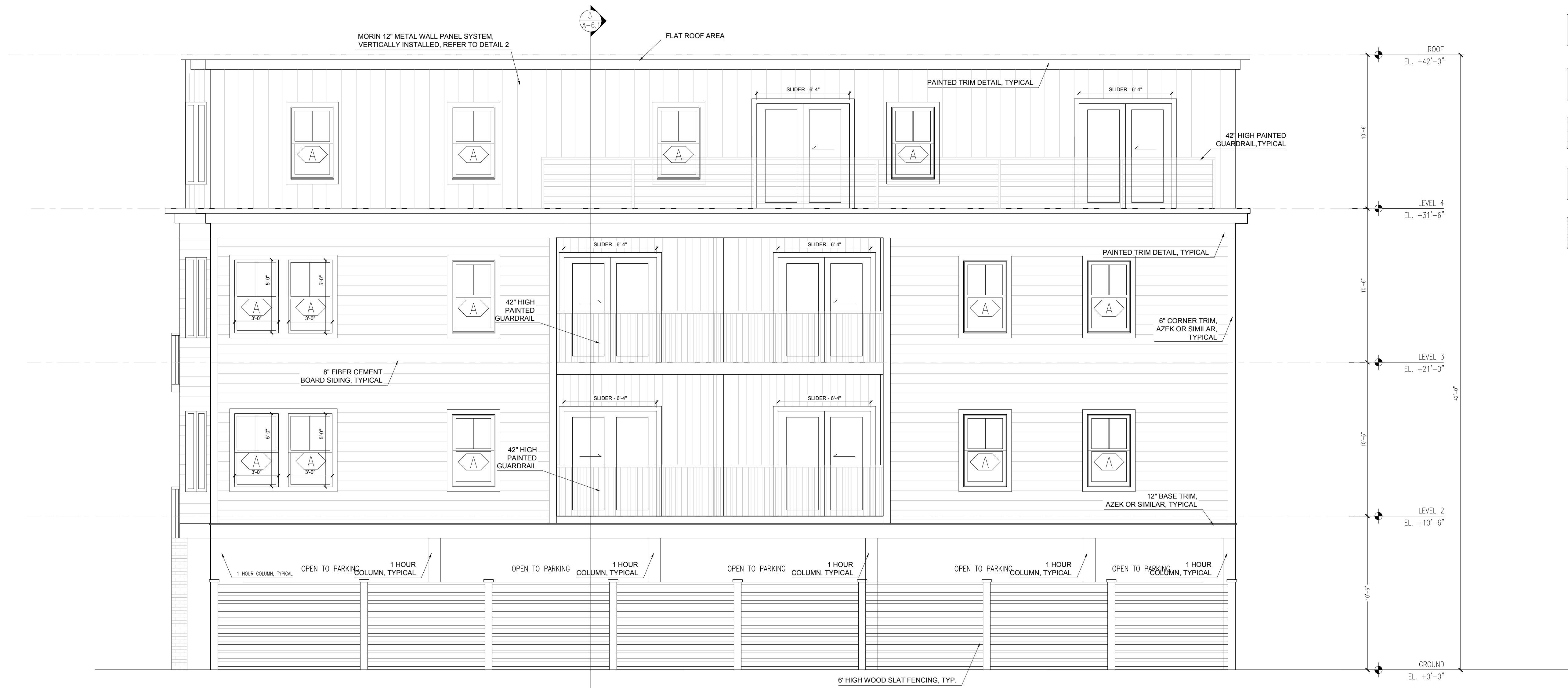
1 REAR OBLIQUE ELEVATION SCALE: 1/4" = 1'-0"
