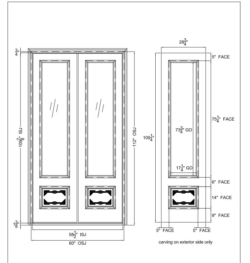
ROUGH OPENING MEASUREMENTS ARE DETERMINED BY ADDING 1" TO THE "OSJ" WIDTH AND  $\frac{1}{2}$ " TO THE "OSJ" HEIGHT
