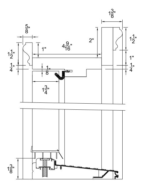
ROUGH OPENING MEASUREMENTS ARE DETERMINED BY ADDING 1" TO THE "OSJ" WIDTH AND  $\frac{1}{2}$ " TO THE "OSJ" HEIGHT
