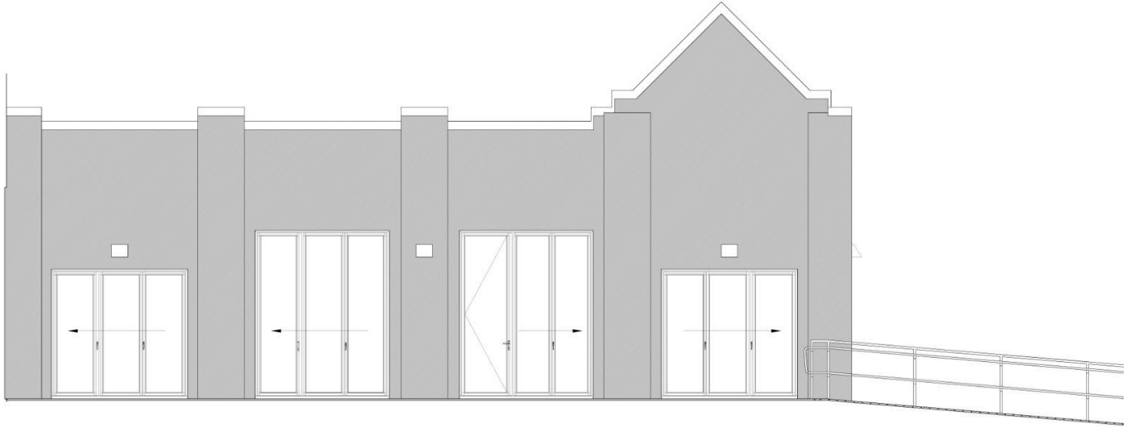
Nanawall SL70 system at four existing openings
