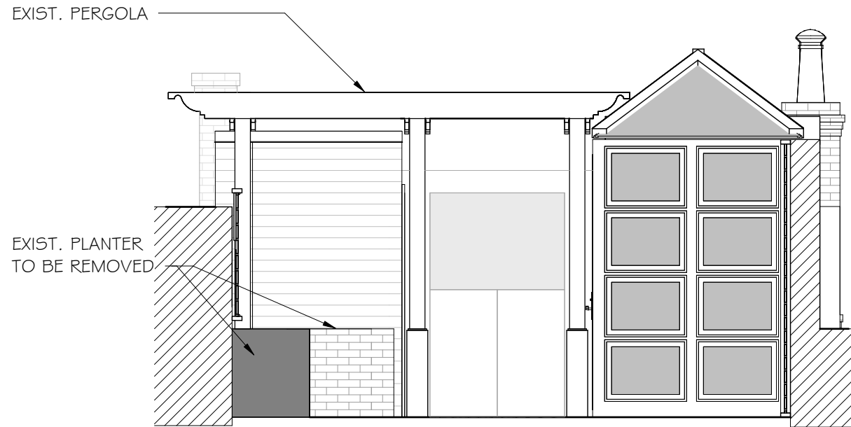
1 ROOF DECK - EXISTING EAST 1/4" = 1'-0"
