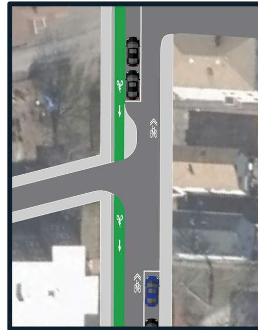
A traffic calming tool that uses offset curb extensions or on-street parking to reduce driving speeds.
