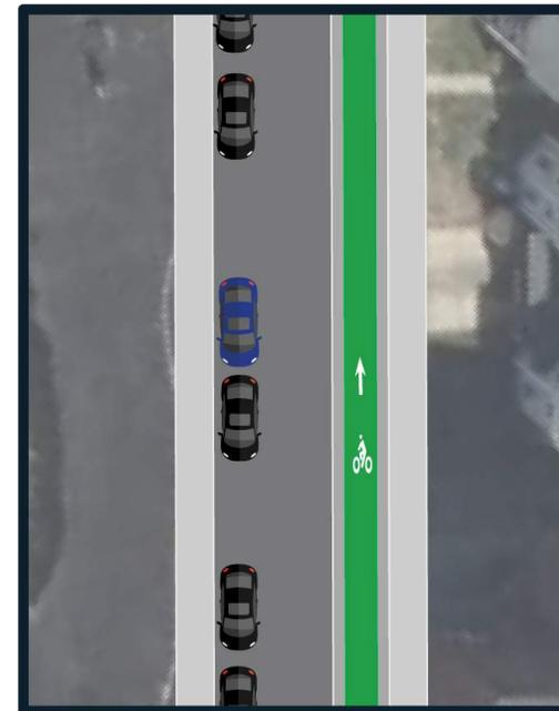
A separated bicycle lane provides both horizontal and vertical separation between people biking and driving. Separation is often provided by flex posts or by raising the bicycle lane to sidewalk level.
