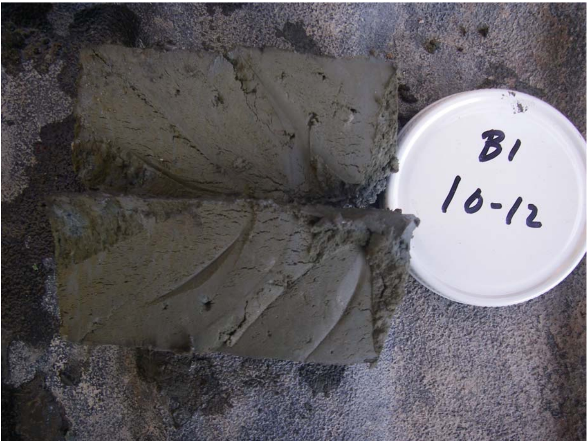
Photo 5: Hard desiccated cohesive silty clay marine sediment in B1 at 11 ft. depth
