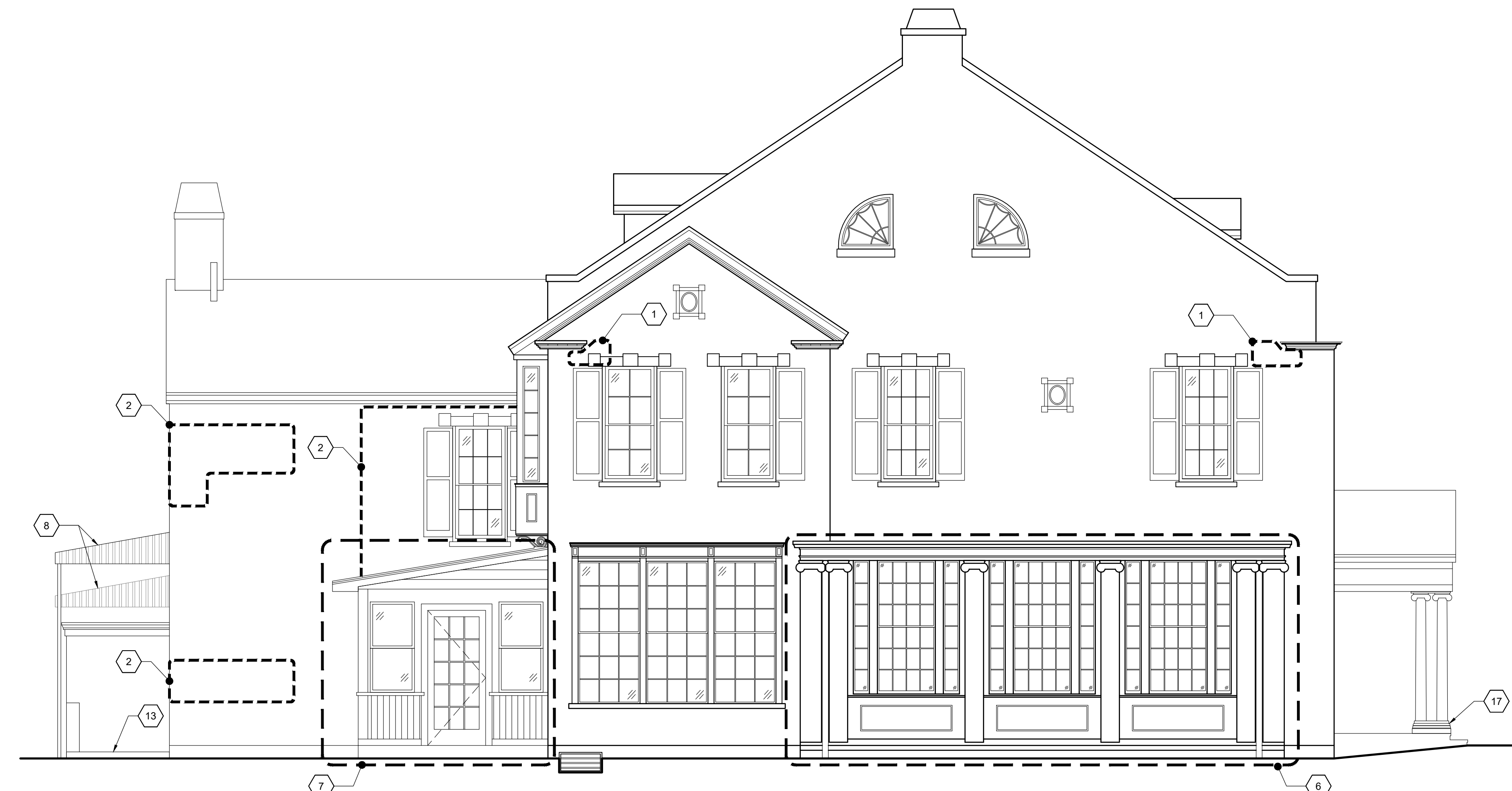
1 NORTH ELEVATION (MORaine STREET) - EXISTING 1/4"=1'-0"
