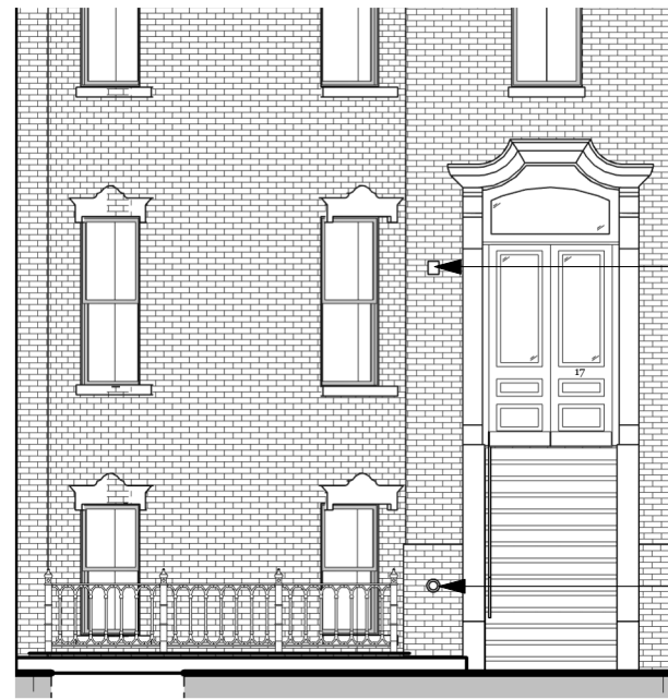
1 FRONT ELEVATION - PROPOSED F.D.C. 1/8" = 1'-0"
