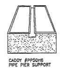
2 TYPICAL CONDUIT ROOF SUPPORT SLEEPER SCALE: NTS
