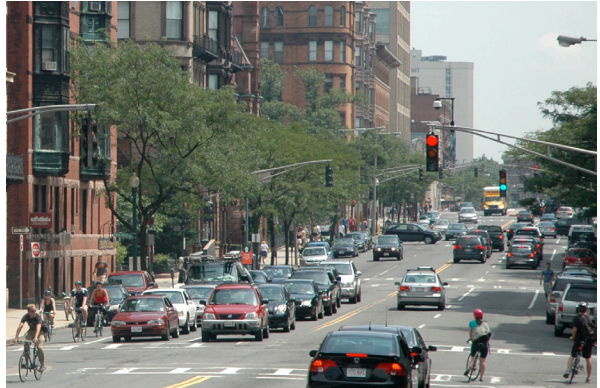
Before Road Diet: Massachusetts Avenue with parking on both sides of the street and two travel lanes in each direction.
