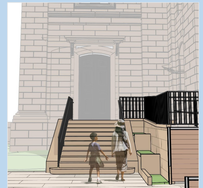
Proposed new brownstone stairs reconstructs the details of the stair but has a compliant top landing
