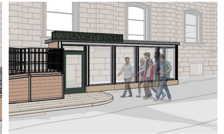
Proposed basement stair enclosure with c-channel steel structure, picture windows and signage.
