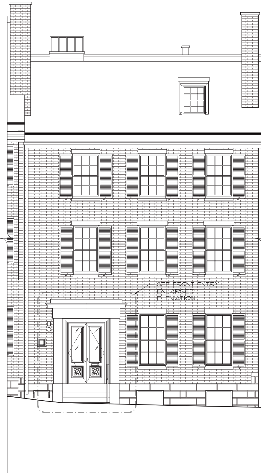
1 FRONT EXTERIOR ELEVATION FULL: 1/4" = 1'-0", HALF: 1/8" = 1'-0"
