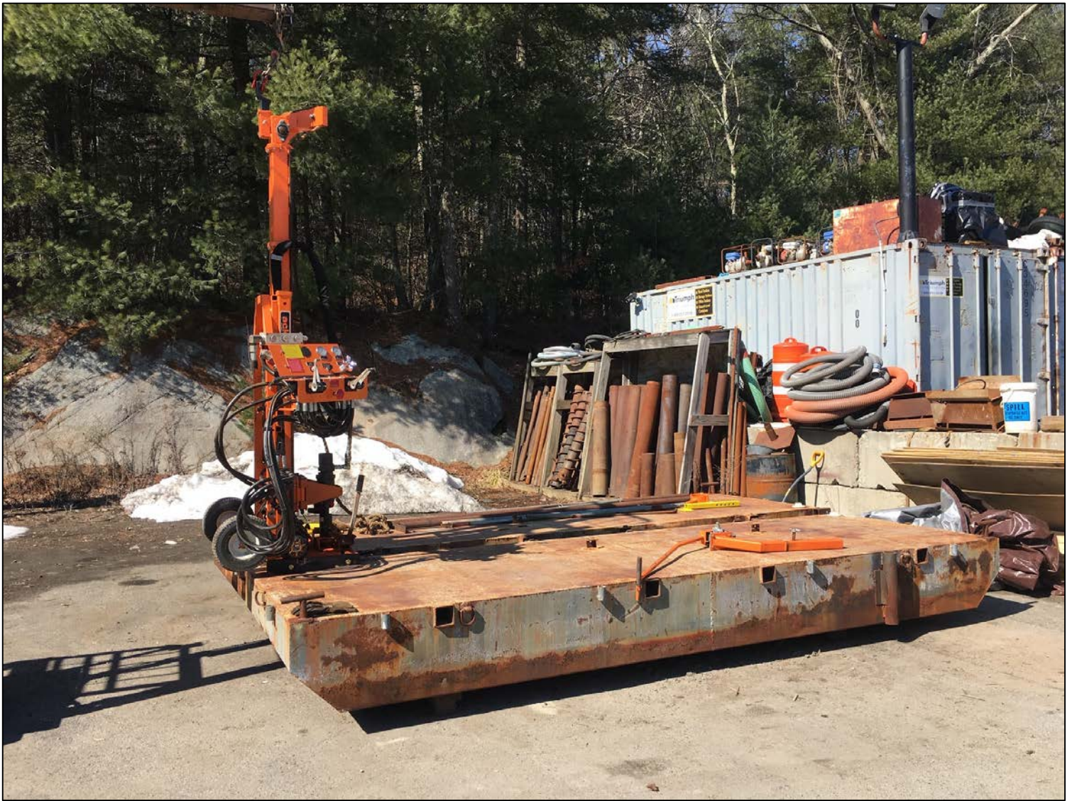
Photo 3: Photo of drill rig on barge similar to what will be used for this sampling effort.
