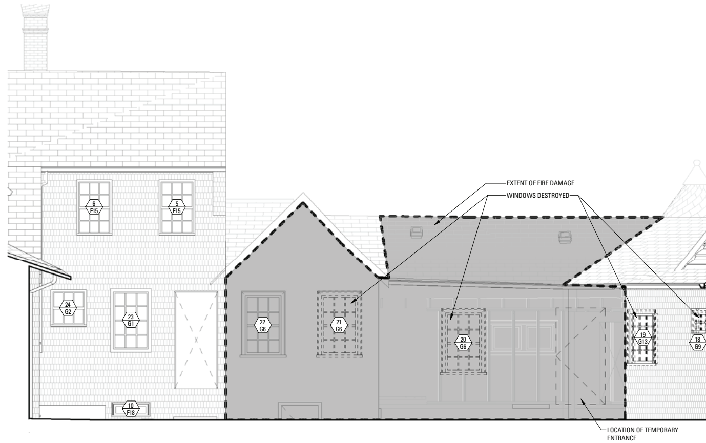
4 BLDG F+G - SOUTHEAST ELEVATION SCALE: 1/4" = 1'-0"
