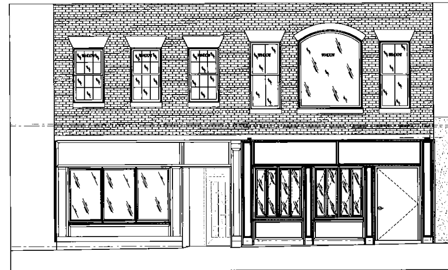
E2 EXISTING ELEVATION ALONG BROAD STREET SCALE: 1/4" = 1'-0"
