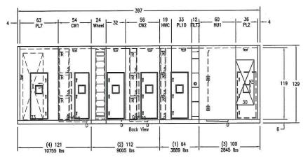
All dimensions shown in inches, Operating weights shown in pounds. Overall unit dimensions do not include lifting lugs, electrical panels, pipe connections, door handles, etc. Panelized Construction Drawing not to scale.
