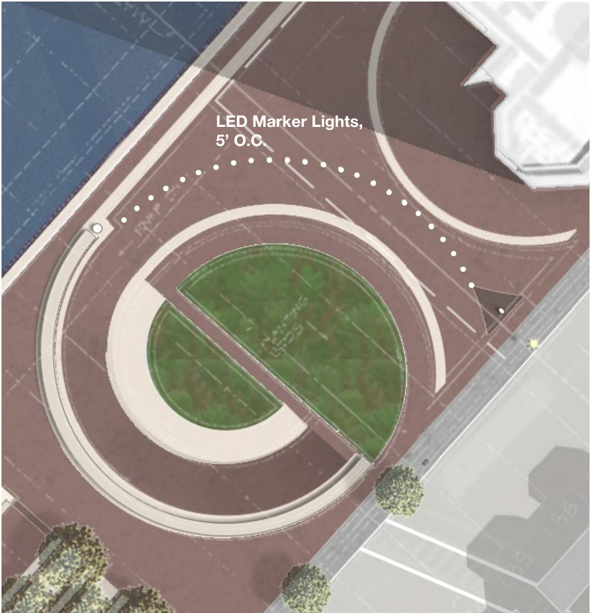
Vehicle Activated Ingrade LED Marker Lights (Activated by exiting vehicles at night and in low-level light conditions only)
