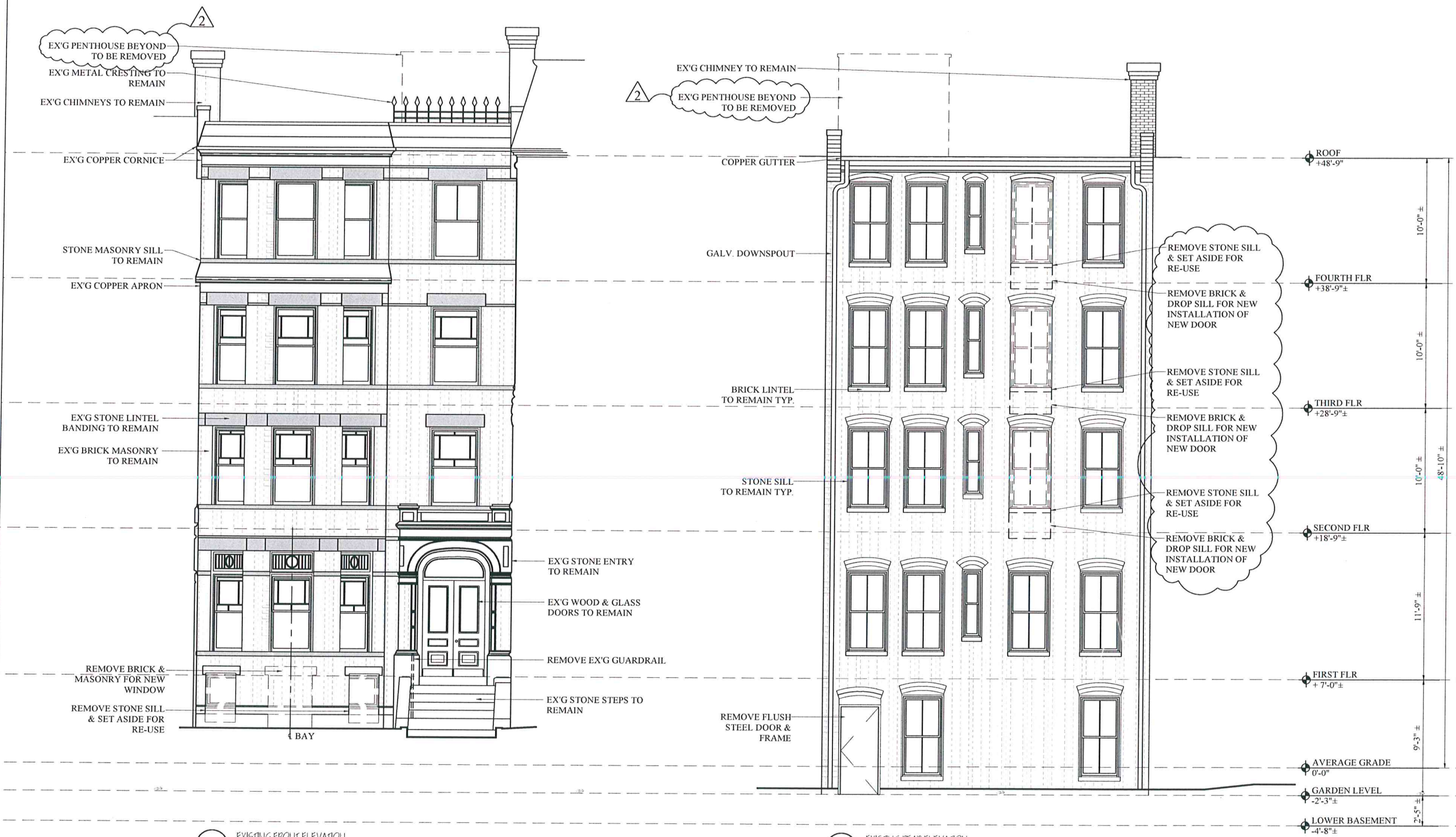
1 EXISTING FRONT ELEVATION 1/4" = 1'-0"
