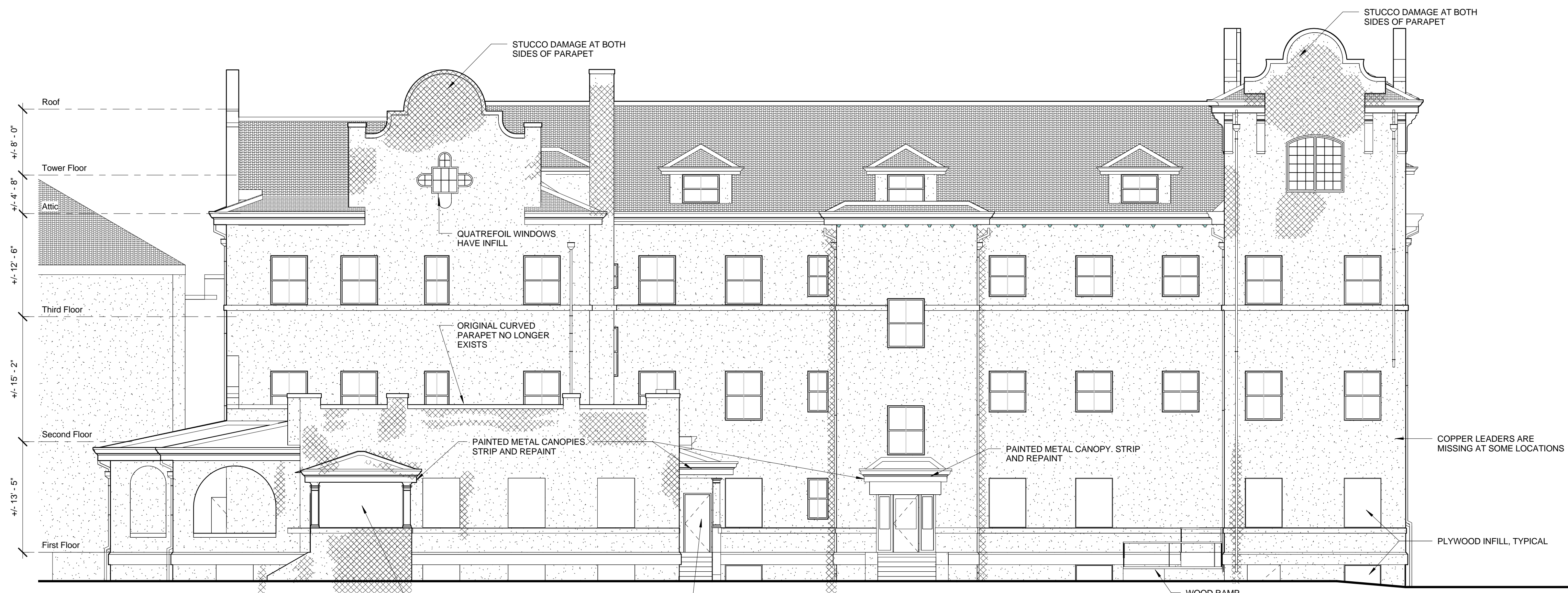
1 Existing West Elevation 1/8" = 1'-0"
