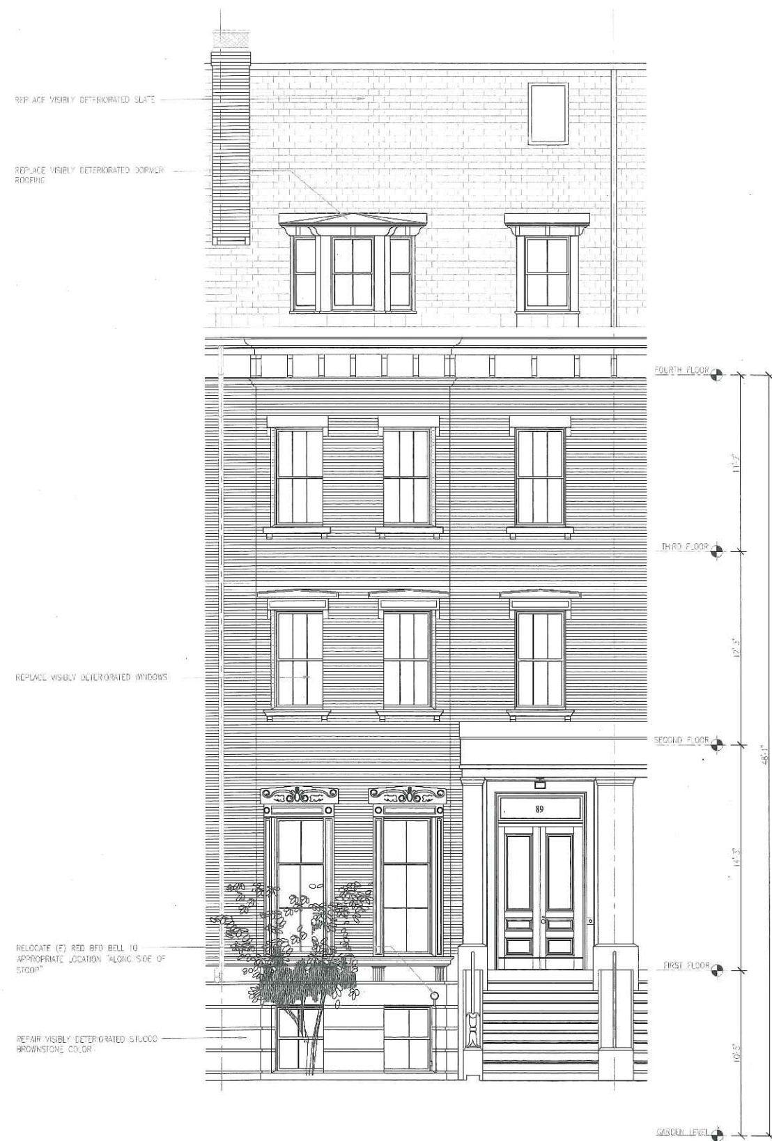
1 EXISTING BEACON STREET ELEVATION SCALE: 1/4" = 1'-0"
