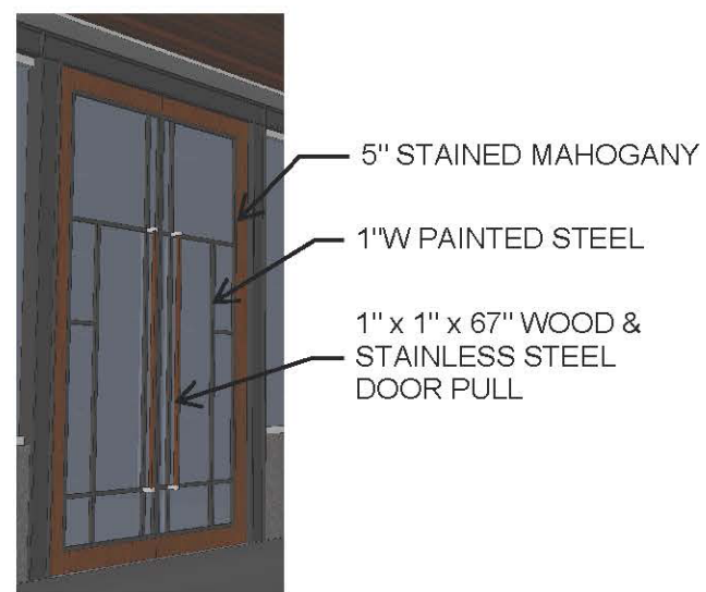
MAIN ENTRY (2) 3' X 10' X 1 3/4" STAINED MAHOGANY AND STEEL DOOR
